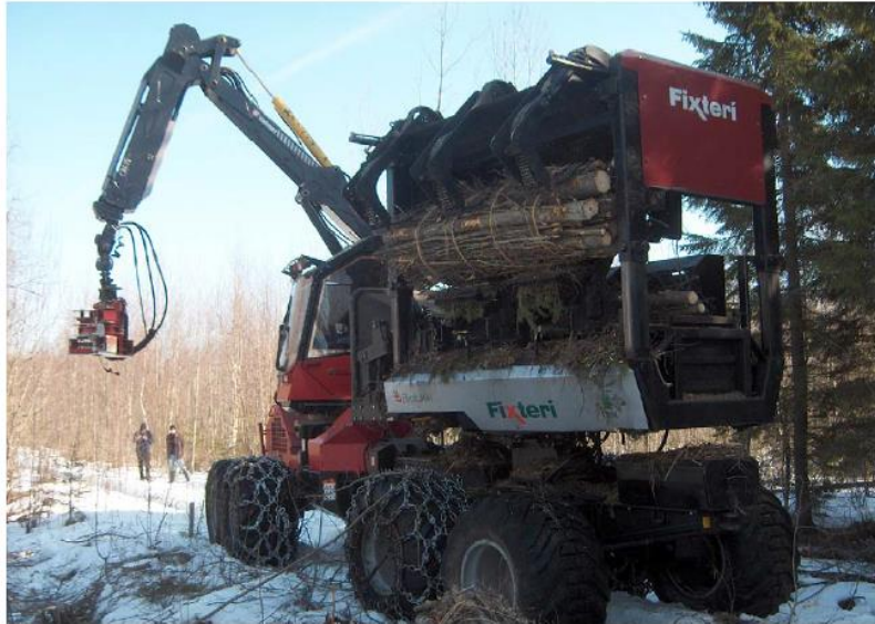
Figure 23. Fixteri whole-tree baler for harvesting pulpwood and energy wood. © Ari Erkkilä.
