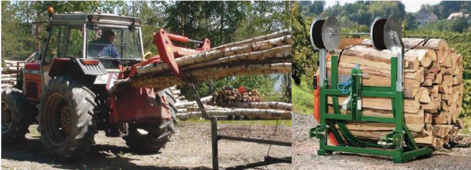
Figure 24. A skidding grapple, which can be used in forming bundles and as an auxiliary tool for bundling of split firewood. © Ari Erkkilä and http://www.posch.com
