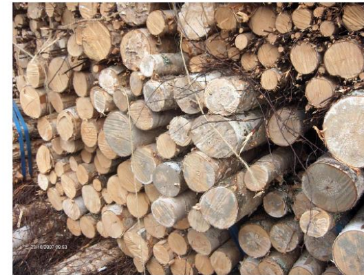
Figure 20. Fungal and mould growth formed on the ends of untreated pieces of logwood. © Ari Erkkilä.
